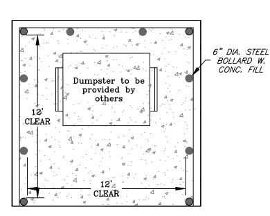
Typical Dumpster Enclosure – Plan N.T.S.
